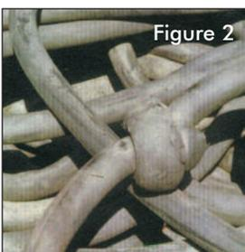
hidden beneath a small mark on the outer jacket. Mechanical damage to inner components also occurs when the cable is bent in a radius far smaller than the manufacturers' recommendations. When dragging cables, be sure to work all kinks, knots, and loops out of the run. Otherwise, the loop will become taut around the cable and end up
