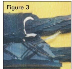
sometimes delicate nature of soft copper stranding and the rubber materials inside the cable. Developing an appreciation for the product capabilities and limitations will go a long way toward reducing mechanical damage. Training on proper bending radius will also be helpful. Large diameter ropes or slings can reduce handling damage.
