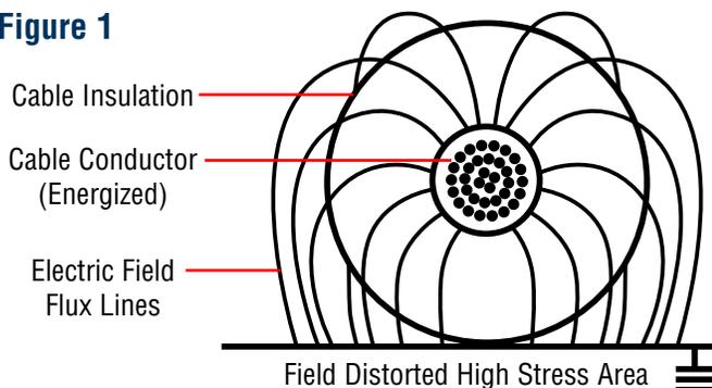
or other contaminates, surface tracking (discharging to ground) can cause cable failures.
