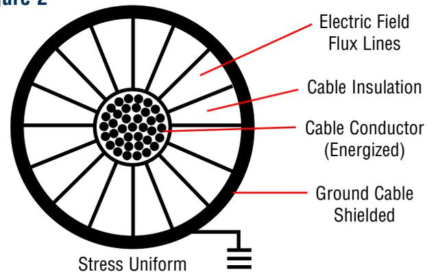
To shield, or not to shield, is a highly charged topic among cable designers, engineers and users. There are many conflicting opinions on the necessity of shielding for different voltage classifications and operational conditions. The following facts (see back page) about non-shielded and shielded cables are universally accepted by cable engineers and Nexans AmerCable.
